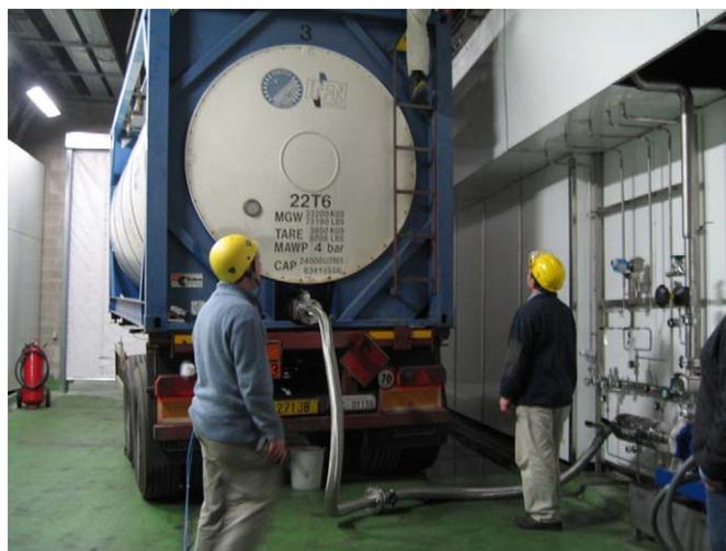
Fig. 8. Tanker truck unloading pseudocumene into the storage area in Hall C at Gran Sasso. The tanker made trips back and forth to Sardinia to bring freshly distilled pseudocumene from Polimeri Europa for the Borexino detector. The tanker is connected to the pump of the unloading station and the pseudocumene is pumped into the 100 m<sup>3</sup> storage tanks in Hall C.
