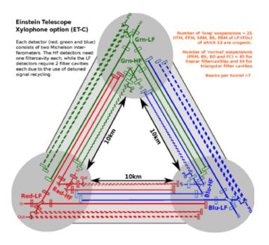
Possible simplified scheme of the ET lay-out. The observatory will be able to host up to three detectors, each composed by one or two interferometers (courtesy S.Hild).
