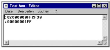
The second file, TEST.HEX, is more relevant because this file holds the commands later programmed into the AVR chip. This file looks like this.
