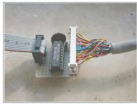
The necessary program algorithm is done by the ISP software, that is available from ATMEL's software download page.
